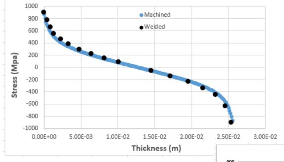
The welded analysis was exactly the same as the machined analysis except the FEM stress distribution input was changed (slightly) from the machined distribution to the welded distribution as shown in the figure on the left.....
