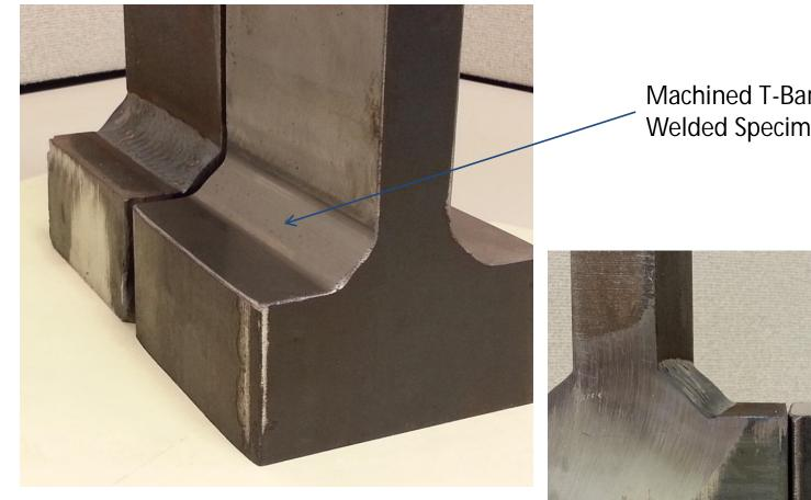
Machined T-Bar Replicates Welded Specimen Geometry
