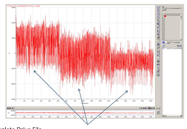
Complete Drive File – 3 Repeats of Transmission, 1 Repeat of Bracket, 2 Repeats of Suspension
