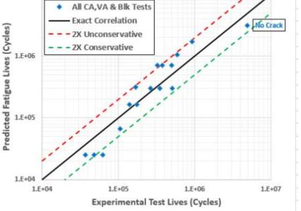
Whole Life Fatigue Life Predictions to *"Failure"* 1)The fatigue life predictions of the welded
