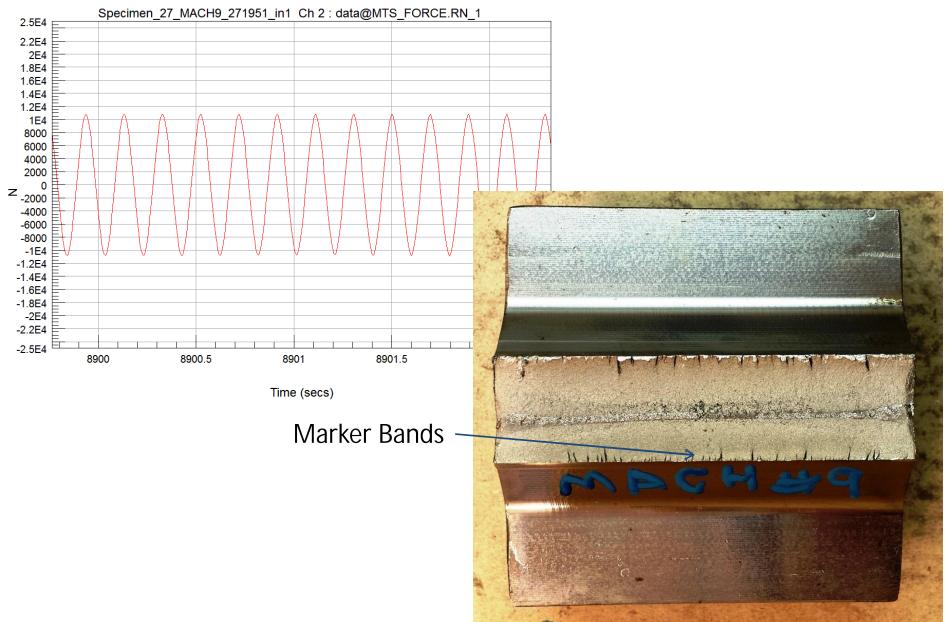
24 kN Max / 24 kN Min, VA, Time History Profile (Trans x3, Brkt x1, Susp x2)
